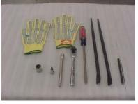
Necessary Tools: 3/8" Drive Ratchet Pry bars (2) Flat Blade screwdriver 6" socket extension 3/8" Gloves 1/4" Hex Allen wrench/socket 1/2" Socket
