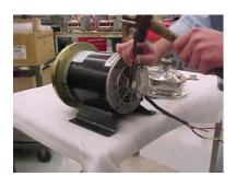
**5.** Remove the Cap at the lead end of the motor. A screwdriver slot will be exposed. Use a screwdriver to stop the shaft from turning.
