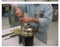
**16.** Check for free rotation then replace the cap at the rear of motor. Reinstall pump/motor into unit.
