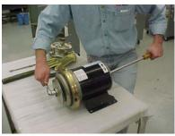
**14.** Replace the impeller lock nut and washer by turning clockwise. Prevent shaft rotation by using a screwdriver on the shaft end screwdriver slot.
