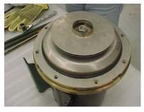
15. Replace the casing and casing screws and tighten finger tight. Finish tightening the cap screws alternately and evenly to approximately 6 ft. lbs. torque. Note: It is imperative that screws be tightened alternately and evenly, as this action centers the cover in the casing, assuring proper alignment. Binding of the impeller in the case and adaptor may occur if the cap screws are not tightened as listed above.
