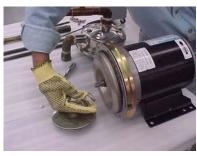
**8.** Remove the spring to the mechanical seal assembly.
