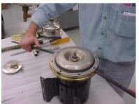
9. With two pry bars 180° apart and inserted between the seal housing and the motor plate adapter and carefully separate the two parts. The mechanical seal assembly will come off of the shaft inside the seal housing. It is not necessary to remove the cast iron disc from the motor.
