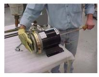
**7.** Remove the impeller by turning counter clockwise. Protect the hand by wearing a glove.
