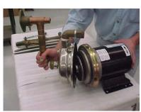
**4.** Remove Casing Screws and Remove Case. Inspect O-ring for wear or damage.
