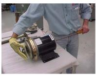
**13.** Thread the impeller onto the shaft by turning clockwise. Protect the hand with a glove. Prevent shaft rotation by using a screwdriver on the shaft end screwdriver slot.
