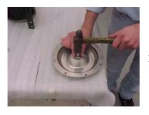
**10.** Using a dowel, push the mechanical seal assembly out of the seal housing from the motor side.
