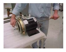
**6.** Remove the impeller lock nut and washers by turning counter clockwise when looking at the front of the pump.
