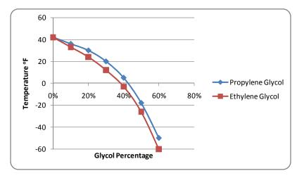
NEVER use automotive glycol in a chiller system as they contain silicone and/or paraffin which over time or due to low temperature operation will plate out or coat the wetted surfaces thereby acting as an insulator and reduce the heat removal capacity and the system efficiency.
