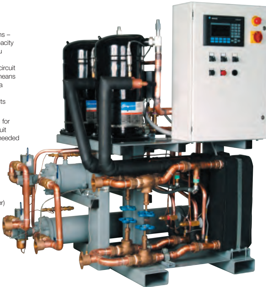
Shown: 30-ton, dual-circuit, water-cooled system with isolation valving and manifolds.
