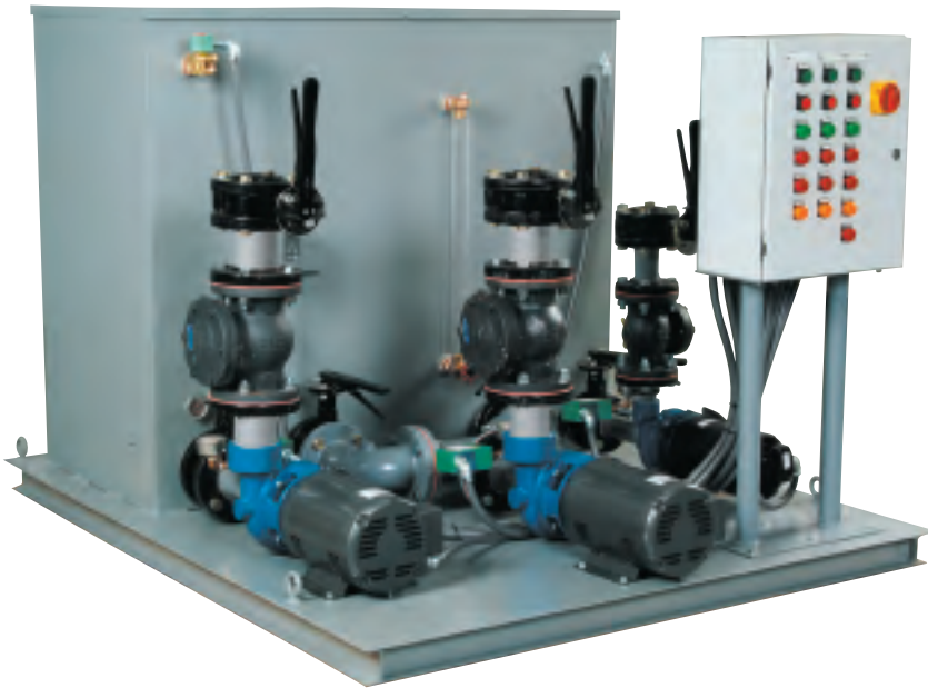
250 gallon carbon steel epoxy-coated pump tank with 3 pump configuration (process, recirculating and backup), with butterfly valves on discharge for flow adjustments and NEMA 4 electrical enclosure
