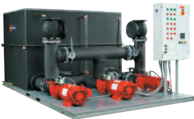
1000 gallon stainless steel insulated chiller pump tank with 3 pump configuration (process, recirculating and backup), showing suction and discharge manifold for ease of plumbing and NEMA 4 electrical enclosure
