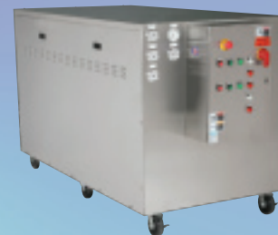
Combination heater/chiller system for clean room environment with all stainless steel cabinetry, NEMA 4X enclosure and custom control integration.
