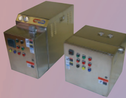
Water systems with NEMA 4X panels. Larger unit has SS louvered panels for wash down resistance. Smaller unit with 2" connections for air sweep to dissipate heat.
