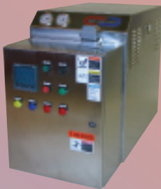
Mokon high temperature and pressure water system used to heat double-walled vessel. Housed in a stainless steel louvered cabinet for wash down resistance with NEMA 4X electrical control panel enclosure.
